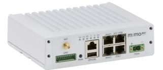
The latest radio in the Mimomax product range, Pyxis can be a stand alone solution or intergrated with the Mimomax Tornado in a multi-tier solution. The Mimomax Pyxis is software programmable over a channel bandwidths of 25kHz and 50kHz.
