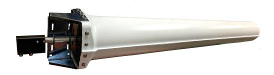
The 700MHz Dual Polarized MiMO Yagi Antenna with Radome is a high gain, premium quality antenna with excellent port to port isolation. Manufactured using high strength 6061-T6 aluminum and anodized for aesthetic and corrosion resistance.
