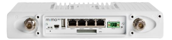
Utilizing MIMO technology, full-duplex communications and high order modulation (QAM256), the Tornado radio can achieve higher rates of data throughput than standard narrowband radios. The result is a better **return on investment** in the spectrum and the ability to run more voice channels over the same link.
